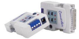
The *icAS/IP*, interface converter allows full conversion between a computer / terminal RS-232 ASYNChronous port and a SYNChronous modem. The icAS/IP conforms to the ITU-TV.22 standard and accommodates the difference in frequency between the asynchronous port and synchronous modem. This unit derives its baud rate automatically from the transmit clock of the modem and operates at data rates from 300 to 19200bps.
